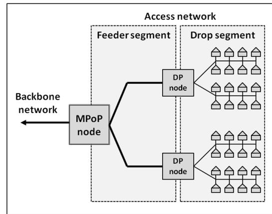
Figure 1 – Fiber access network architecture
