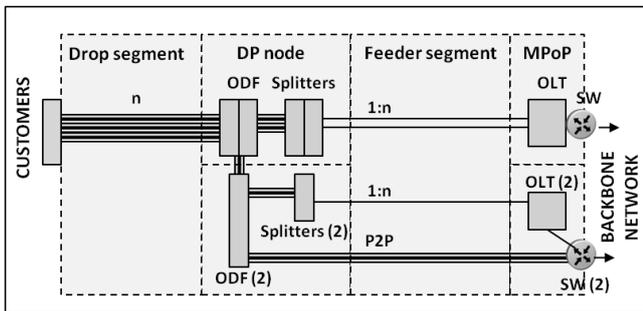
Figure 3 – Access to P2MP FTTH network at DP (splitters) node
