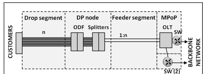
Figure 4 – Access to P2MP FTTH network – OLT level bitstream
