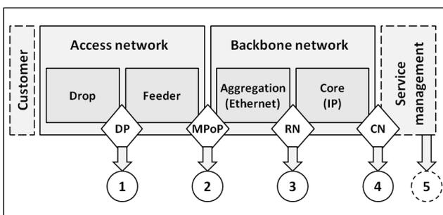
Figure 2 – Reference FTTH network architecture with interconnection points
