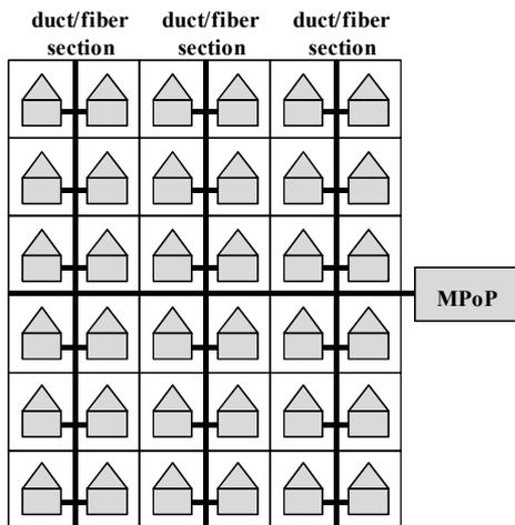
Figure 1 – Square geometric model of duct/fiber network, bold lines represent duct/fiber sections
