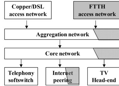
Figure 4 – FTTH model in relation to operator's existing network (new and upgraded network parts are shaded)
